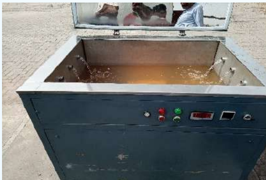
Hot Water Treatment Plant Fabricated under PSDP PESC at Gourmet Sugar Mills Farm
