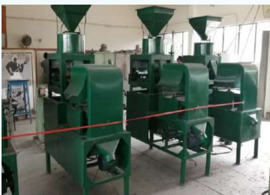
Ispaghool processing machinery developed by AEI, NARC, Islamabad
