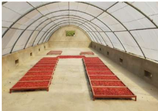
Solar tunnel dryer and one solar-cum-gas fired dryers
